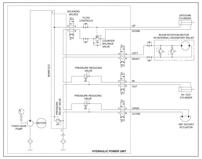
Figure 5A Hydraulic Schematic
