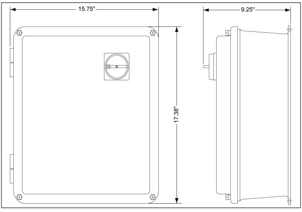
Figure 6B Standard NEMA 12 Disconnect Control Panel Detail
