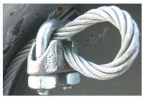
Image 9 – Folding and clamping cable
